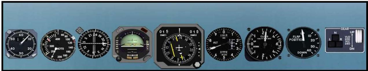
We have now reached 15NM on the DME. We are at 9,700' MSL. I have tuned the HSI to a course of 041 for when we cross over the LAX VOR. Until then, we will not be using it. We will navigate DIRECT to the LAX VOR using the RMI, which is pointing down, directly to the VOR.
