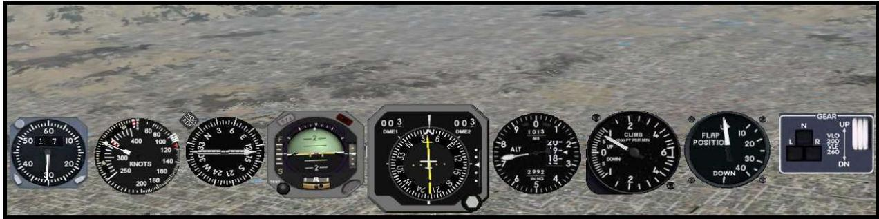
We are now over the LAX VOR – the RMI has swung to the side and is turning around. The HSI says we are “on course” but this is a lie – we are over top of the VOR and therefore the HSI cannot pick up the signal. The mileage to the DME says 3NM, but this is because we are 3 NM **ABOVE** the VOR in altitude. We will maintain a heading of 041° and when the signal picks up, we simply get on the radial and track outbound.
