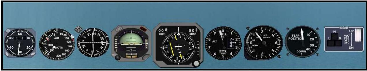
We have turned to a heading of 235° and are climbing out. Note that the DME is nearly 8 NM and that we are maintaining an indicated airspeed below 250 KIAS, since we are below 10,000' MSL
