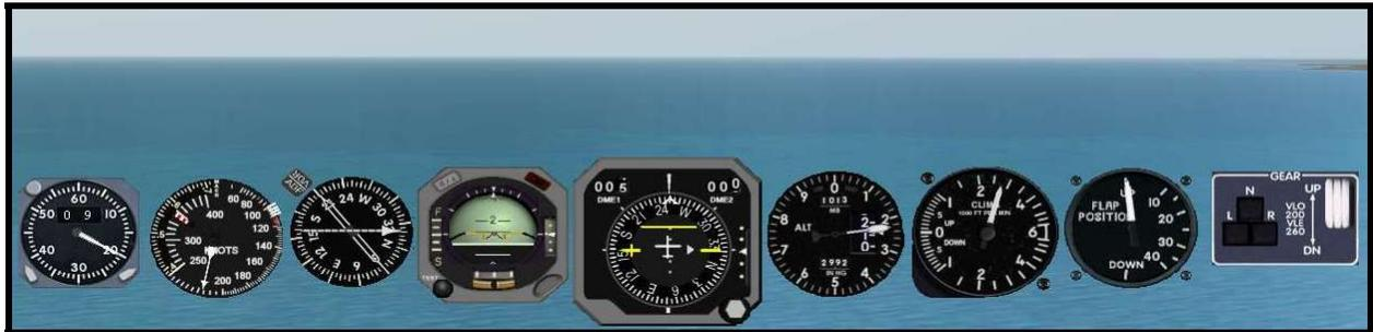
We are flying a heading of 250° and are climbing out. Note that the SMO R-160 is programmed into the HSI.
