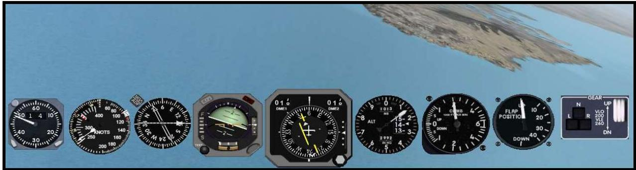
We are still in the turn, but as you can see with the RMI, it is pointing to about 035° to where the LAX VOR is located. We will level the wings when the RMI for the LAX VOR is pointing straight up and accelerate at that point.
